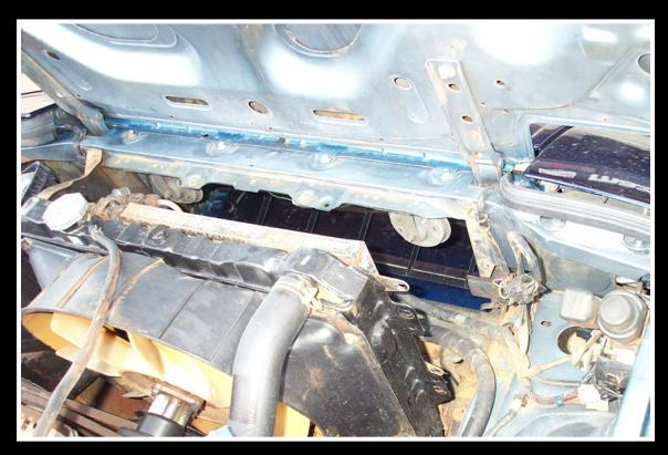
Here we are with top and right supports removed and the coolant overflow reservoir moved out of the way.
