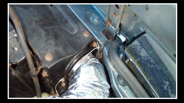
Secure this spot here with the 2nd 4 1/2" hose clamp, and now your Insulated Cold-Air Intake is complete. For additional heat soak protection, a heat shield over the intake manifold is a bonus. Enjoy your new, colder-fed engine!
