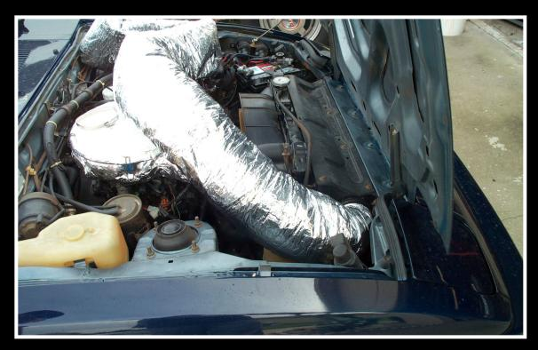
Here we've attached the reinforced end to figure out how much additional ducting well need. Most stores don't sell the length you'd want, but around 2 feet seems to be the appropriate number. Better to have too much, than too little.
