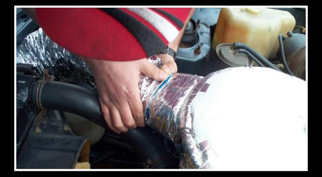
Upon placing this end around the air cleaner housing, you'll find that it's not likely to hold on it's own. Bring in the first 4 1/2" hose clamp!
