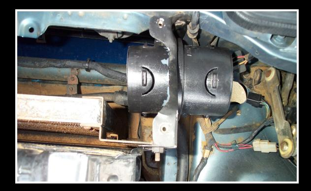
Here we have placed the right radiator support back in place. From experience, we would recommend that you put the 90° bend on first, or at a minimum, place it in front of the radiator to install once the support is in place. Trust us - we've been here and done that.
