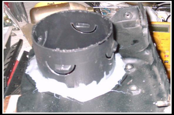
After drying, fit the elbow onto the sleeve - in our application we had to remove 1/4" off of the end to get the elbow to lock in place. Below you can see the fitted and attached apparatus. Notice the downward angle on the elbow This is where the cold air will enter this system. Future revisions may include a megaphone-style scoop if it indeed proves beneficial - Bernoulli seems to suggest it should.
