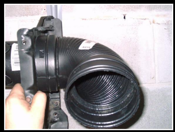
Here we are test-fitting the sleeve, 90° bend and the radiator cover. Once satisfied, use epoxy to glue the sleeve into the radiator support.
