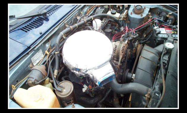
Here's the reinstalled INSULATED air cleaner housing. Simply insulating this would go a long ways towards preventing heatsoak - but why stop there?
