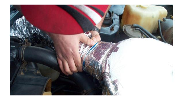
Upon placing this end around the air cleaner housing, you'll find that it's not likely to hold on its own. Bring in the first  $4 \frac{1}{2}$  hose clamp!
