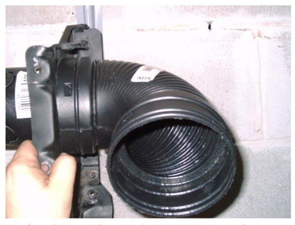
Here we are test-fitting the sleeve,  $90^{\circ}$  bend and the radiator cover. Once satisfied, use epoxy to glue the sleeve into the radiator support.
