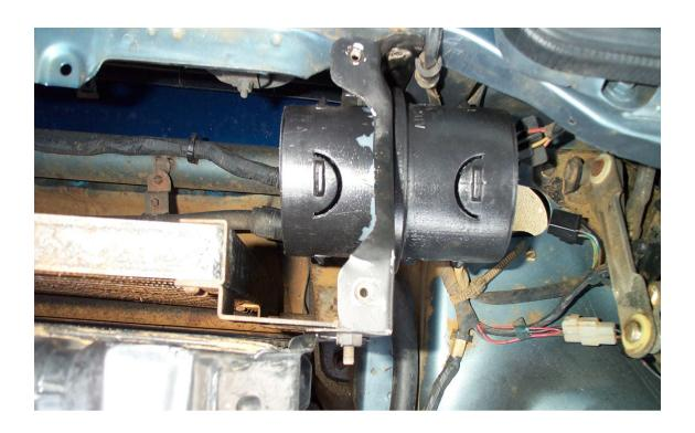
Here we have placed the right radiator support back in place. From experience, we would recommend that you put the 90° bend on first, or at a minimum, place it in front of the radiator to install once the support is in place. Trust us - we've been here and done that.
